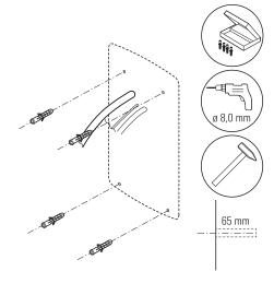
6 Screw the mounting rail into the two upper mounting points using the two TX30 plug screws and the Torx screwdriver.
