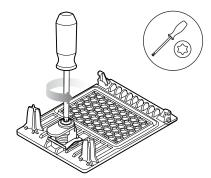
5 Push the locking cylinder out of the guide of the RCCB flap with the screwdriver.
