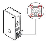
2 Loosen the four screws with a Torx TR 20 screwdriver and pull the charging flap off the wallbox.
