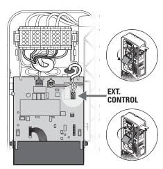
After establishing the electrical connection of the control cable, the remote disconnection function must be activated via the ABL Configuration App. To do this, please refer to the sections starting on page 38.
