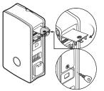
4 Close the RCCB flap and lock it with the key.
