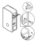
2 Flip the toggle switch of the RCCB to the **0** position.
