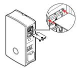
4 Check the replaced RCCB flap to ensure that it moves freely and then lock it with the key.
