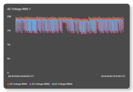
For a better overview and allocation, the voltage curve for each conductor is displayed in its specific colour. The vertical range extends from zero to the nominal grid voltage, the horizontal timeline is linked to the time frame of the Control Pilot Status.
