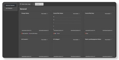
If the selected charger is online (connected to COSMOS via the Internet), the page displays the charger's **Live Telemetry** data and can also be used for diagnosis of errors in the charging system.
