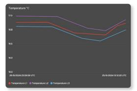
For a better overview and allocation, the temperature curve for each conductor is displayed in its specific colour. The vertical temperature range is adapted to the maximum and minimum temperature of all three conductors, the horizontal timeline is linked to the time frame of the Control Pilot Status.
