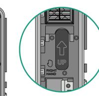
**3.2** Hold the charger, aligning the three lower tabs, then attach the wallplate flaps to the charger.
