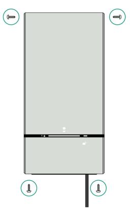
Remove the **three screws** (Torx Ø4 x 12mm) from the HMI module, then fold it down carefully until it hangs vertically.
