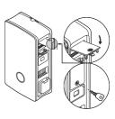
4 Open your domestic power distribution box, disconnect the wallbox's power supply cable from the electricity grid via the MCB, secure the MCB against being switched on again and close the distribution box
