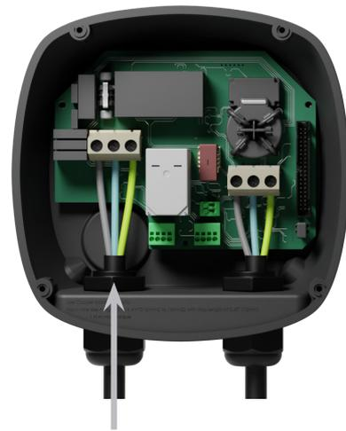
When using this opening for the communications cabling, first remove the screw plug. Use a wrench to hold the interior lock nut while unscrewing the plug using a flathead screwdriver from the bottom (exterior) side of the plug.
